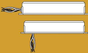
Single-flex units mount onto the junction box or driver compartment and wiring runs to the test accessories via flexible conduit.
