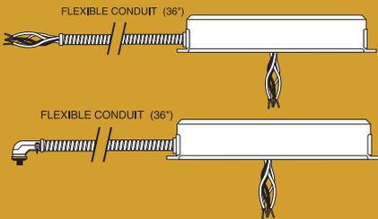
Slim-line units (available for Constant Power units only) feature a 1.2 inch profile for installation within the narrow and shallow compartments of LED strip fixtures.
