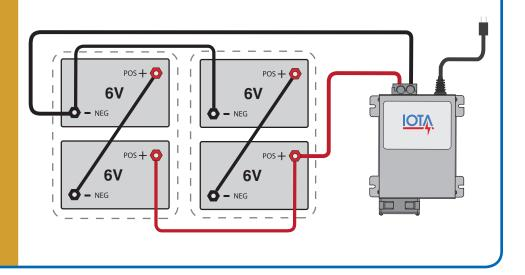
Note that for optimal battery bank and charging performance, the batteries in the bank should be of the same manufacturer and model, as well as the same AH rating, age, condition, and state of charge [SOC]. For additional assistance with using IOTA DLS chargers for your 6-volt battery applications, contact our Technical Services team at 1-855-363-9527 or visit www.iotaengineering.com/services.
