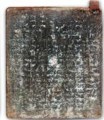
Two common maintenance practices that contribute to sulfation are storing batteries in an uncharged condition and undercharging. Both of these conditions can be prevented by using smart charging technology to safely maintain stored batteries at full charge.
