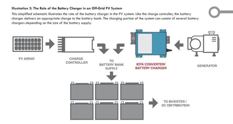
condition and stimulating the mixing of the electrolyte solution\*. Using AC power from the generator, the IOTA IQ4 Smart Controller enables the IOTA DLS Series Charger/Converter to automatically deliver these four charging stages.
